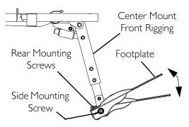
FIGURE 6.18 Adjusting the Footplate Angle - After 2/14/07
